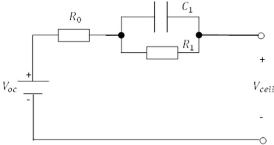
Fig. 1. First order electrical model of the cell
