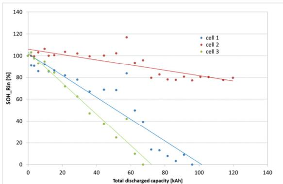
Fig. 3.  $SOH_R$  vs total discharged capacity
