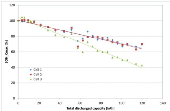
Fig. 2.  $SOH_C$  vs total discharged capacity
